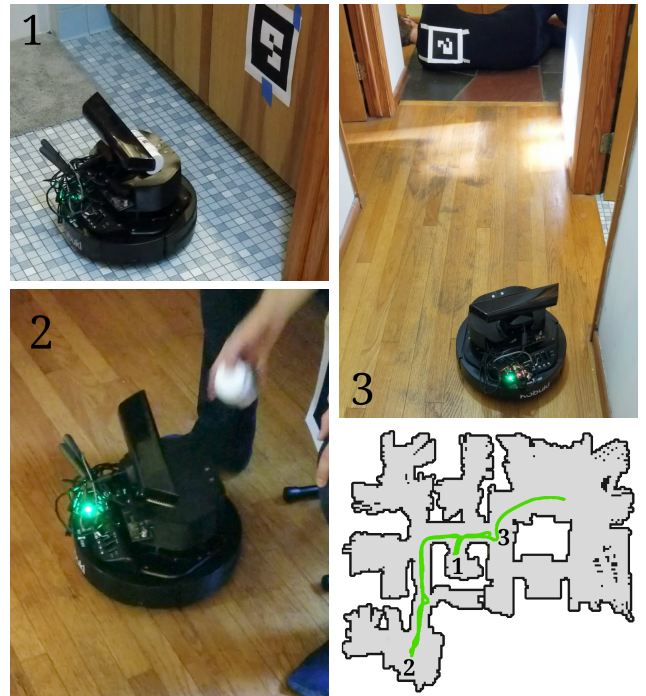
Figure 4: Experiments with the home healthcare robot using this policy network in the real household shown above. Three highlights are shown: (1) medicine retrieval for task t_1 , (2) medicine delivery completion with transfer t_1 \rightarrow h \rightarrow t_2 , and (3) interruption of cleaning task t_2 by detecting a fall with task f_i and calling for assistance.
