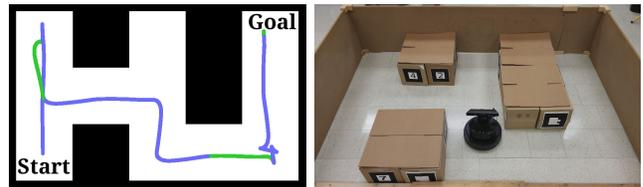
Fig. 2. Robot experiment. Path: FSC (blue), belief (green) actions.
