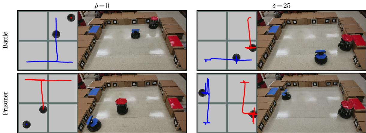
Figure 3: Experiments with CCP on two real robot platforms. Battle Meeting (top row) and Prisoner Meeting (bottom row) are shown with slack  $\delta=0$  (left column) and  $\delta=25$  (right column) for both. The paths traversed by robots “Alice” (blue) and “Bob” (red) over the entire execution are shown as well. For each slack allotment, the robots adapt their policy to work together to satisfy the group task and/or complete their individual box-pushing tasks.
