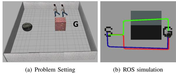
Fig. 2. An illustrative example of a robot navigating in a building, showing the problem setting (left) and its corresponding ROS simulation with black regions denoting obstacles and shaded region denoting human locations (right).  $S$  denotes start location and  $G$  is the goal location. Green line denotes the trajectory computed using determinization, red denotes optimal trajectory, blue denotes that of 0/1 RM.
