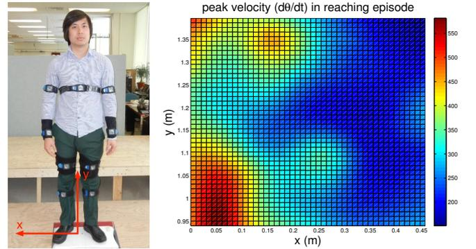
(a) On-body IMU sensors deployed on the subject’s body (b) Computed peak velocities during the reaching episodes; the profile plane is 30 inches away from the human subject
