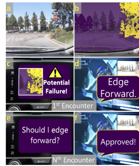
Figure 2: Competence-aware prediction of failures and integration of learned model into planning and execution.
