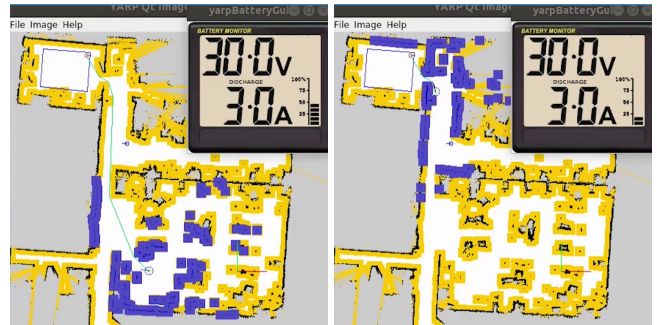
(a) Battery level above 30%. The robot is reaching the destination. (b) Battery level at 25%. The robot keeps moving to the destination. The response property is violated.
