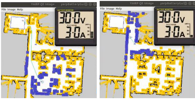
(a) Battery level above 30%. The robot is reaching the destination. The safety property is satisfied. (b) Battery level below 20%. The robot is reaching the recharging station. The safety property is violated.
