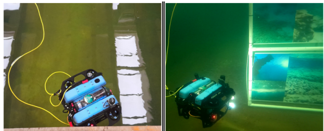
Figure 1: Dora , BlueROV2 operated as an AUV in real applications. The exploration scenario counts with multiple points of interest that require inspection. Dora uses an automated planning system to perform tasks that depend on the AUV sensors and actuators.
