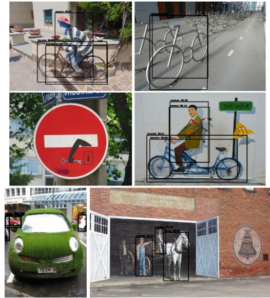
Figure 5: YOLOv3: some unsuccessful cases. (Top-left) Sculpture mistaken for a person on bicycle (Top-right) bike parking confused for bicycle; (centre-left) stop sign not detected; (centre-right) mural with a person on a bicycle classified as real; (bottom-left) undetected car with grass texture; (bottom-right) mural containing cart and people identified as real.
