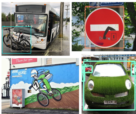
Figure 6: Faster R-CNN: sample successful results. (Top-left) Bus with bicycle mounted in front; (top-right) modified stop sign; (bottom-left) mural with a cyclist; (bottom-right) car with grass texture.
